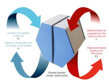
The enthalpy heat exchanger can be ordered separately or later; after a very simple installation, the entire unit is upgraded with advanced technology.
