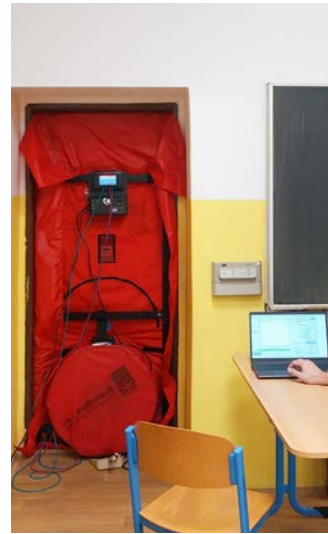
Airtightness measured by Blower Door test
