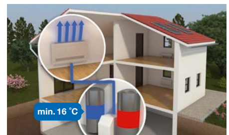
SUMMER heat pump (dry cooling)
