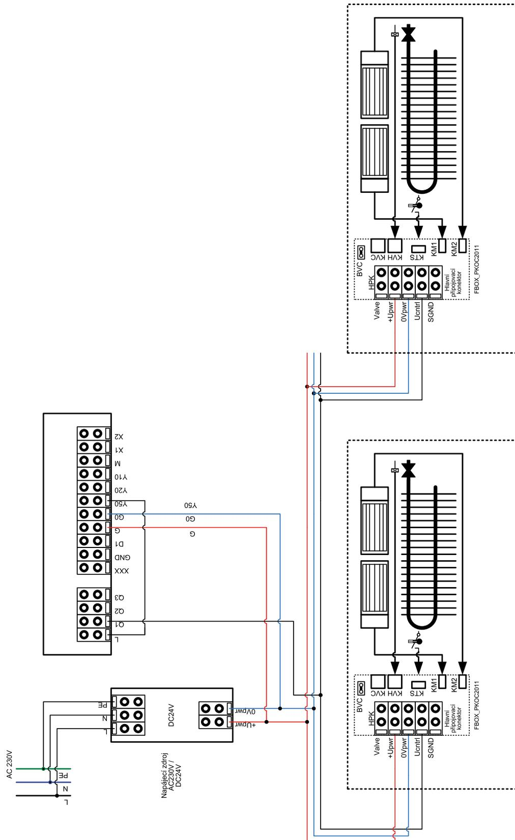
**Note:** Standard regulation is not equipped for independent control of valves (thermal drives) as for 4-tube systems (PKWOC).
