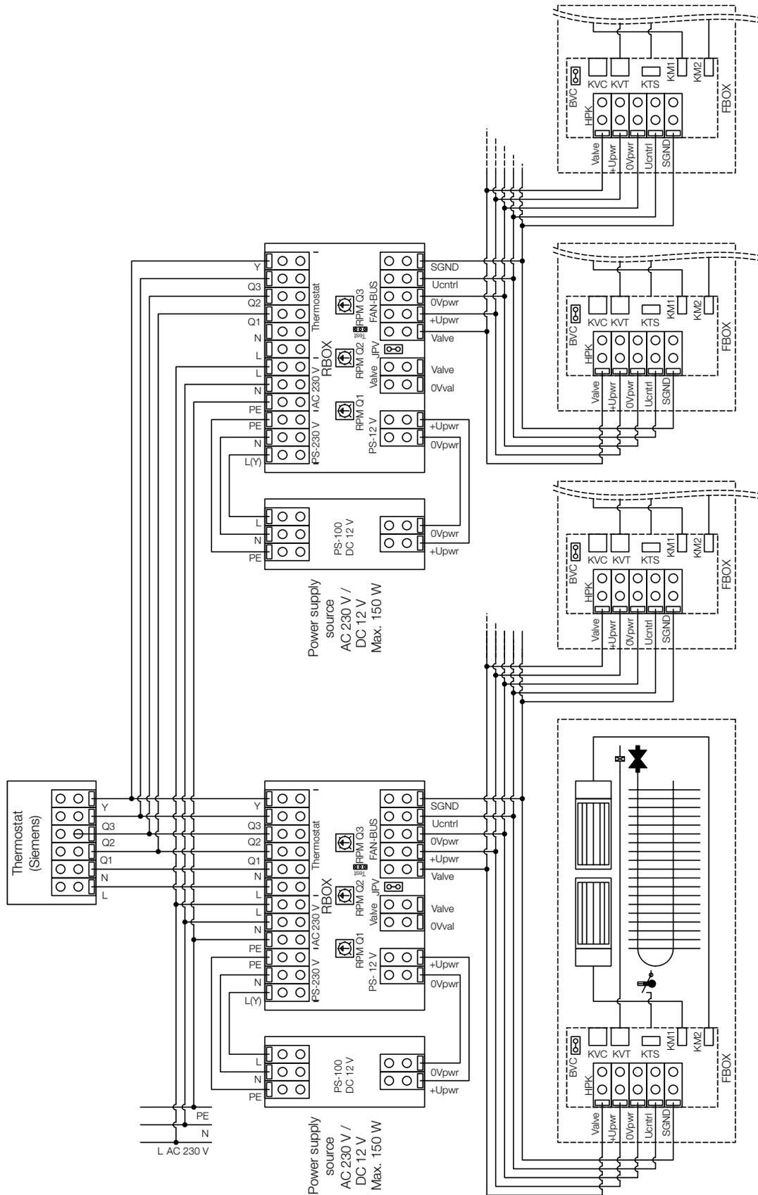
Connection diagram for 24 V DC regulation of LICON OC convectors (PKOC, PKBOC, PKIOC, OLOC, OKIOC), two-pipe system
