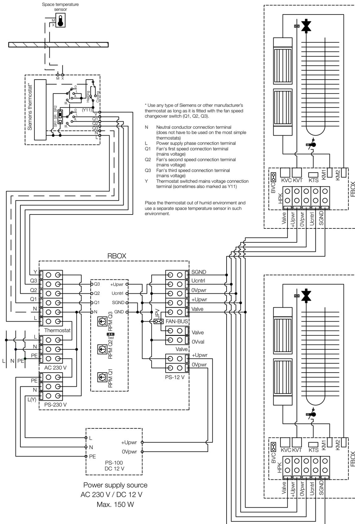
Connection diagram for 12 V and 24 V DC regulation of LICON OC convectors (PKOC, PKBOC, PKWOC, PKIOC, OLOC, OKIOC) – BMS control (Building Management System)
