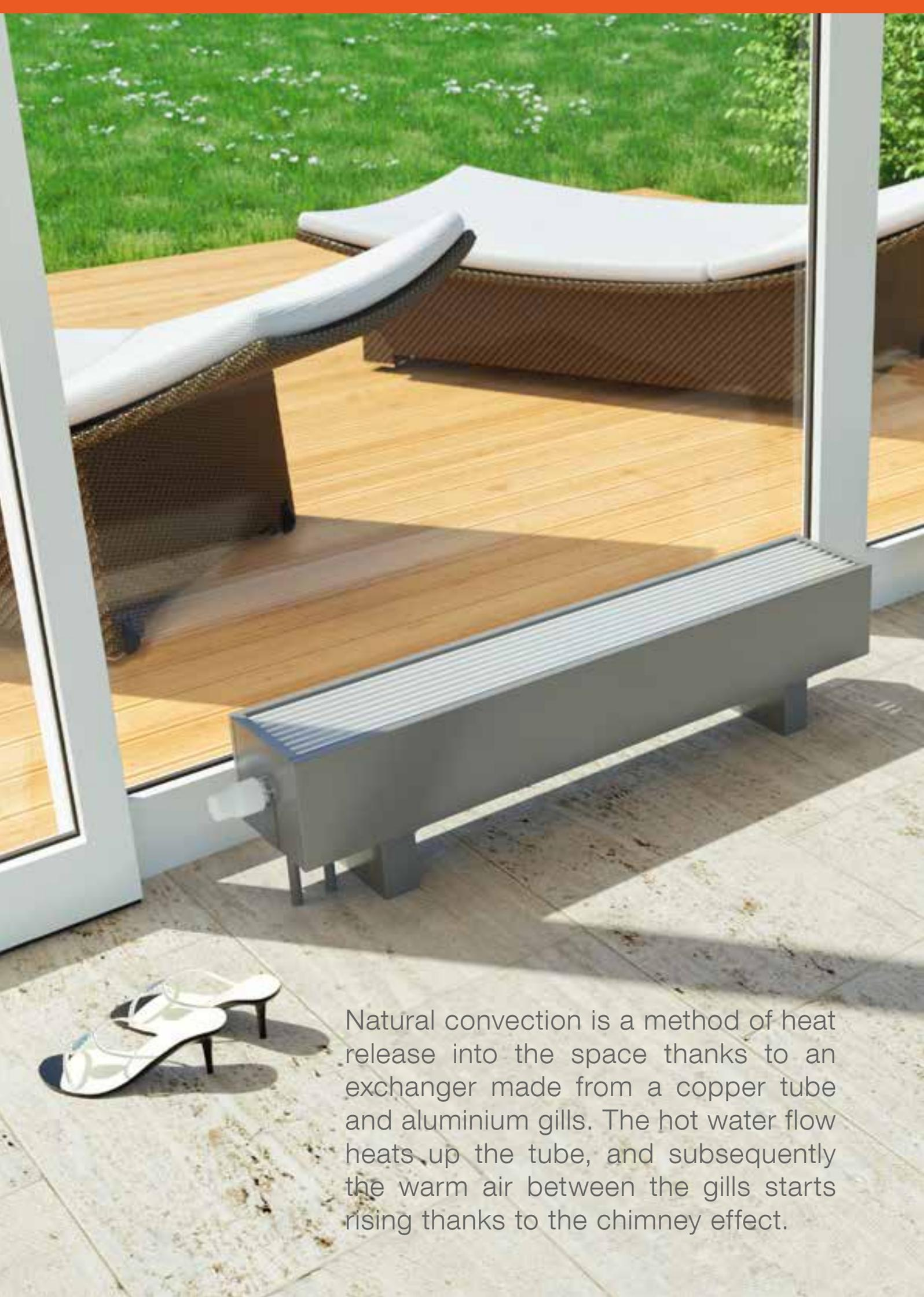
Natural convection is a method of heat release into the space thanks to an exchanger made from a copper tube and aluminium gills. The hot water flow heats up the tube, and subsequently the warm air between the gills starts rising thanks to the chimney effect.
